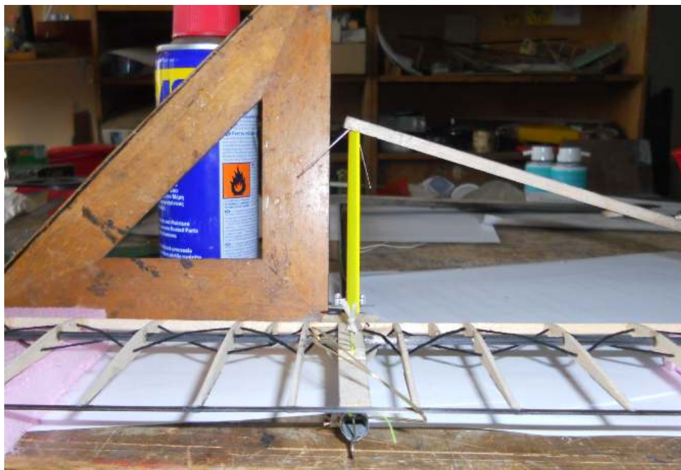
Gluing the fin (laser alignment)
